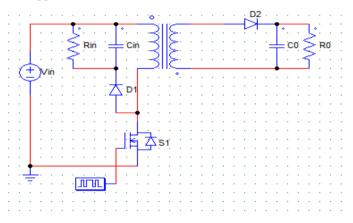
Figure.19 Circuit Diagram of Flyback Converter
