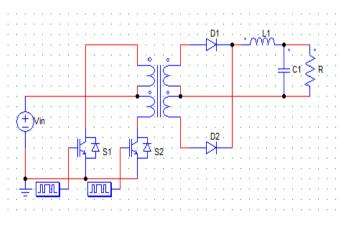
Figure.20 Circuit Diagram of Push Pull Converter
