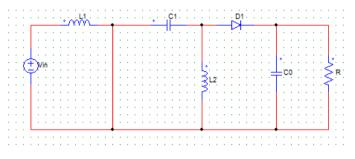
Figure.3 Operation 2 of Sepic Converter, i.e., Switch is in OFF state
