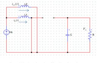
Figure.32 Device 1 Operation of Two Phase Boost Converter
