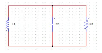
Figure.18 Stage 2 Operation of Buck Converter, i.e., Switch is in OFF state
