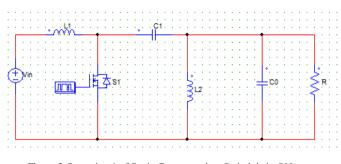
Figure.2 Operation 1 of Sepic Converter, i.e., Switch is in ON state
