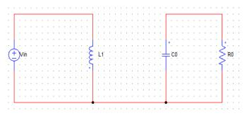
Figure.14 Operation 1 of Buck-Boost Converter, i.e., Switch is in ON state
