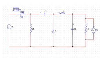
Figure.7Representation diagram of Zeta converter
