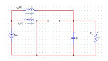
Figure.34 Device 3 Operation of Two Phase Boost Converter
