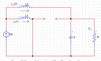
Figure.33 Device 2 Operation of Two Phase Boost Converter
