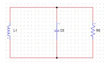
Figure.15 Operation 2 ofBuck-Boost Converter, i.e., Switch is in OFF state
