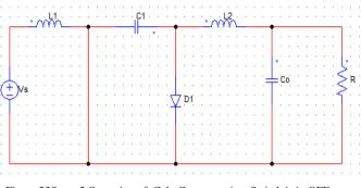
Figure.23Stage 2 Operation of Cuk Converter, i.e., Switch is in OFF state
