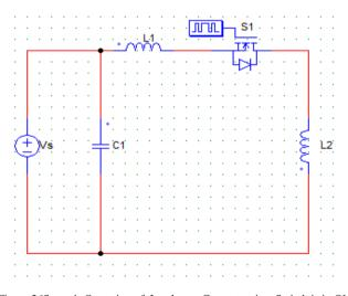
Figure.26Stage 1 Operation of Landsman Converter, i.e., Switch is in ON state
