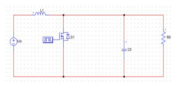
Figure.11 Operation 1 of Boost Converter, i.e., Switch is in ON state
