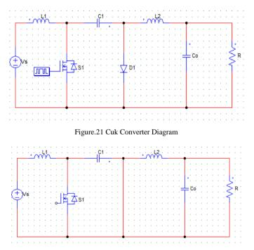
Figure.22Stage 1 Operation of Cuk Converter, i.e., Switch is in ON state
