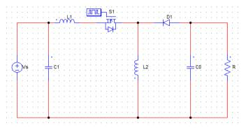
Figure 25. Landsman Converter Diagram
