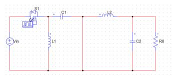
Figure.5 Operation 1 of Luo Converter, i.e., Switch is in ON state
