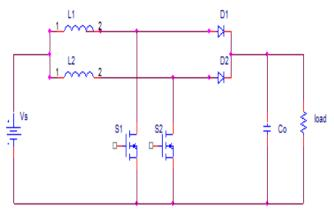
Figure.31 Two Phase Boost Converter Diagram
