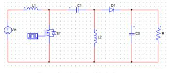
Figure.1 Graphic diagram of Sepic Converter
