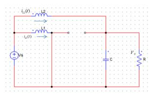
Figure.35 Device 4 Operation of Two Phase Boost Converter
