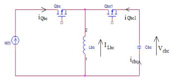
Figure. 36 Equivalent Circuit of Bidirectional DC-DC Converter.
