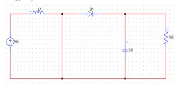
Figure.12 Operation 2 of Boost Converter, i.e., Switch is in OFF state
