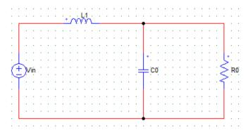
Figure.17 Stage 1 Operation of Buck Converter, i.e., Switch is in ON state
