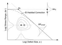
Figure 3 Kitagawa diagram and propagation threshold
