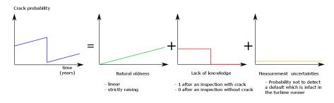
Figure 4 Components of degradation
