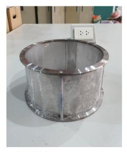
Figure 2 0.4 mm sieve in a rice grinde
