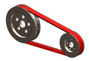
Fig no. 4.2.4 Belt and pulley Assembly
