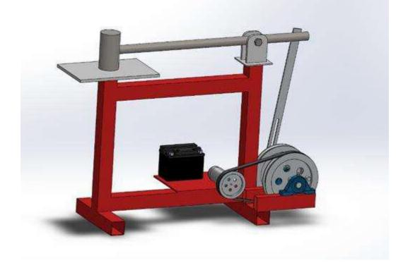
Figure 1.1.2 Simple Electric Hammering Machine
