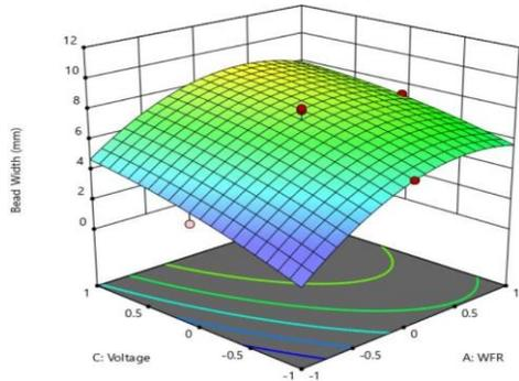
**Fig. 7.** Effects of V and WFR on BW.
