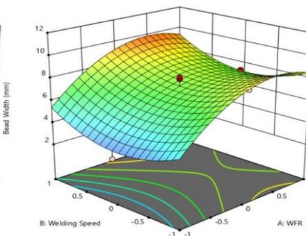
**Fig. 8.** Effects of WS and WFR on BW.
