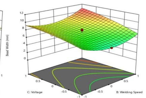
**Fig. 9** Effects of V and WS on BW.
