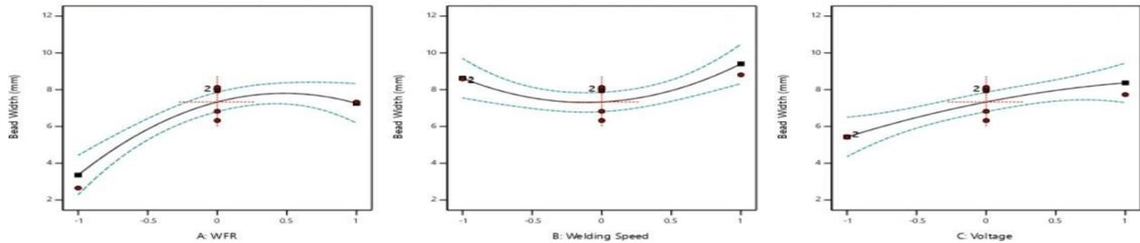
Fig. 4. Direct effect of input parameters on BW.
