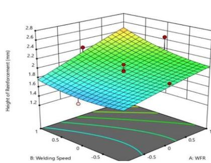
**Fig. 10.** Effects of WS and WFR on HOR
