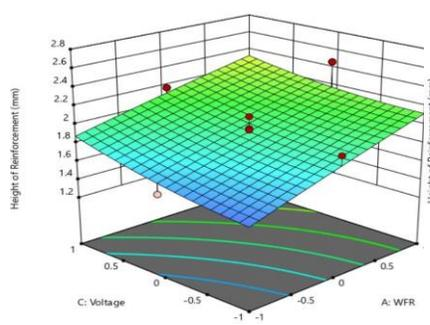
**Fig. 11.** Effects of WFR and V on HOR
