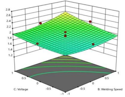
**Fig. 12.** Effects of WS and V on HOR
