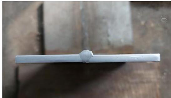
**Fig. 3.** Weld test piece (Etched specimen).
