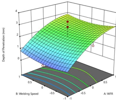
**Fig. 13.** Effects of WS and WFR on DOP
