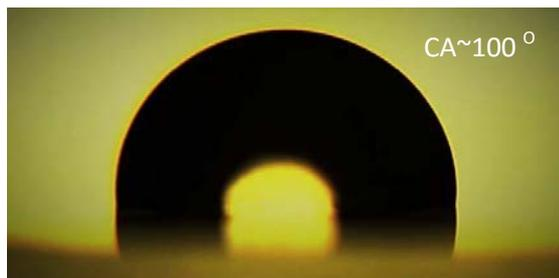
Fig. 2: Water droplet in a hydrophobic surface treated with hydrophobic agent
