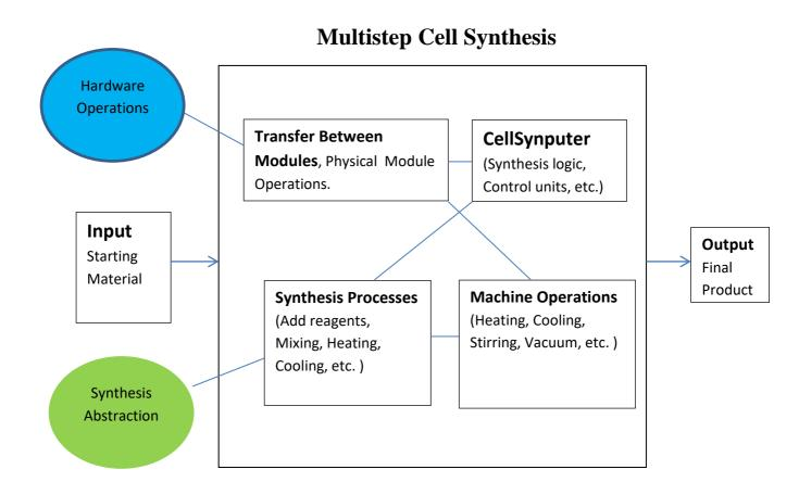
Figure 4. CellSynputer Operational Architecture
