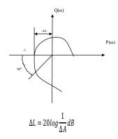
Fig. 4. Amplitude-phase characteristics of the "open" system of the machine adopted into the automation system.
