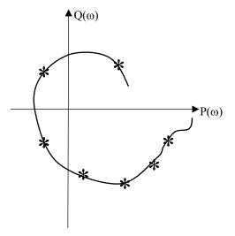
Fig. 3. Amplitude-phase characteristics of the machine adopted into the automation system determined on the basis of the measured amplitude spectrum and the calculated phase spectrum.
