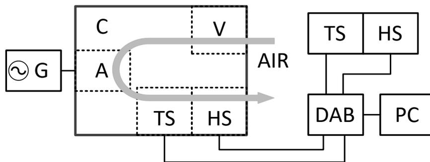
Figure 1 - Block diagram of a calorimetric apparatus for measuring antenna efficiency
