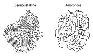
**Figure2**. [Semi-Crystalline polymer and Amorphous polymer (Take note of the entanglements between the polymer chains) [19]
