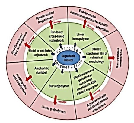
Figure 4. polymers architecture prepared using degradable initiators [46].
