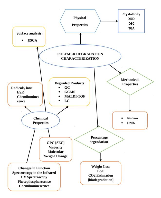
Figure 9: Techniques for characterising polymer degradation in general [30].
