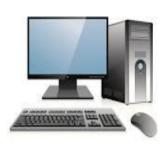
The *electronic machine* is made up of memory unit, Arithmetics logic unit, processor unit, input unit and output unit. The processor unit is made up of data path and control components.
