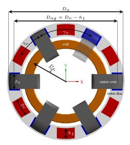
Fig. 3: Axial view of one phase stack of disc rotor TFM
