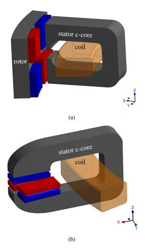
Fig. 5: One pole pair of TFM (a) cylinder rotor - M1; and (b) disc rotor - M2  $\,$
