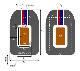
Fig. 4: Cross-section view of c-core
