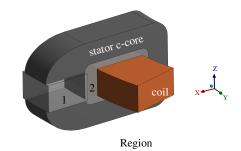
Fig. 9: FEA model to simulate end winding leakage and fringing flux inductance
