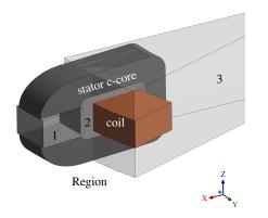
Fig. 10: FEA model to simulate fringing flux inductance
