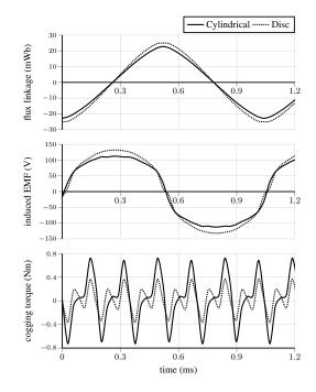
Fig. 6: FEA results of cylindrical rotor and disc rotor TFM at no-load
