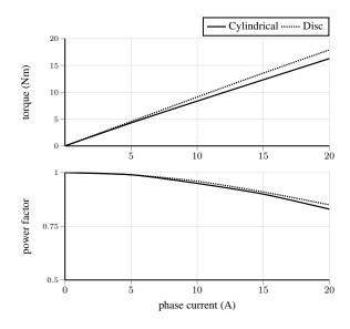
Fig. 7: Effect of armature current in cylindrical rotor and disc rotor TFM
