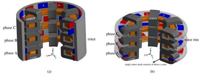
Fig. 1: Cut-section view of TFM (a) cylindrical rotor; and (b) disc rotor
