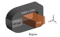
Fig. 8: FEA model to simulate magnetizing inductance
