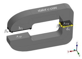
Fig. 2: Cut-section view of single c-core
