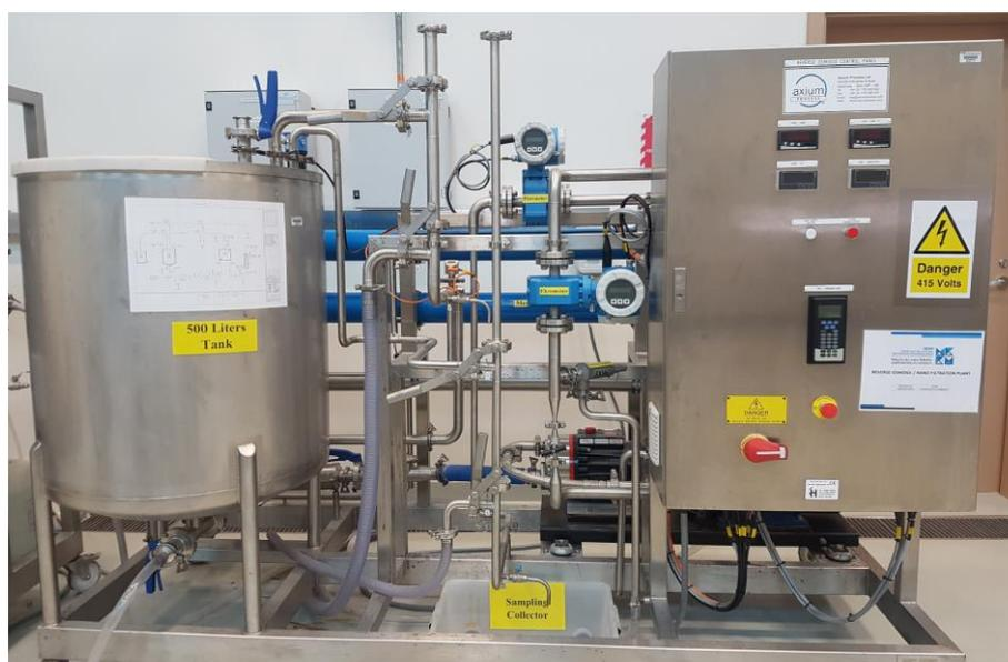
Figure 1. Reverse osmosis test rig
