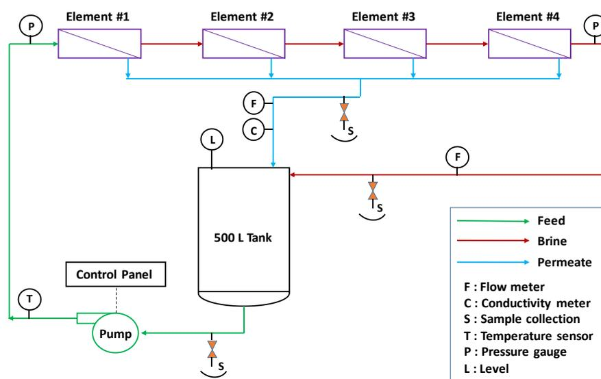
Figure 2. Process flow diagram of RO test rig
