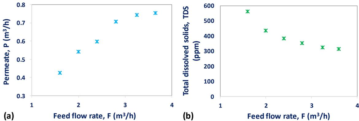
Figure 3. (a) Permeate flow rate and (b) salinity with respect to feed flow at 55 bar
