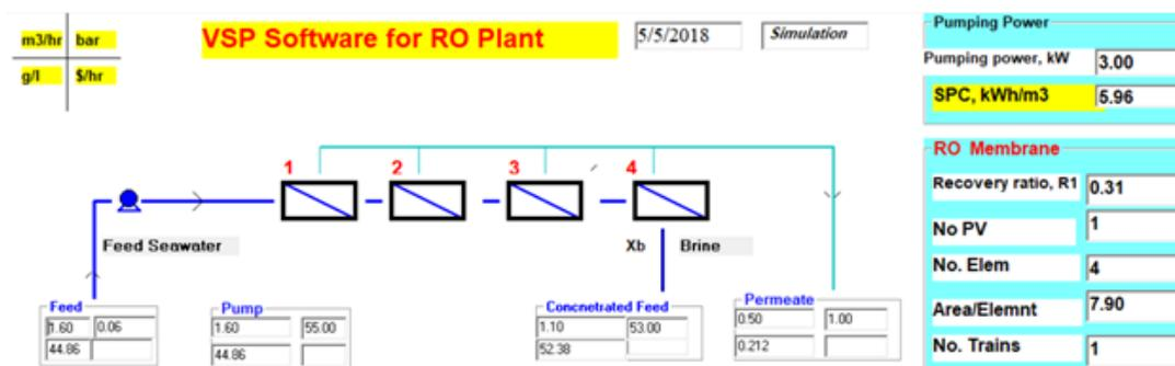
Figure 7. Four elements RO configuration in VSP software
