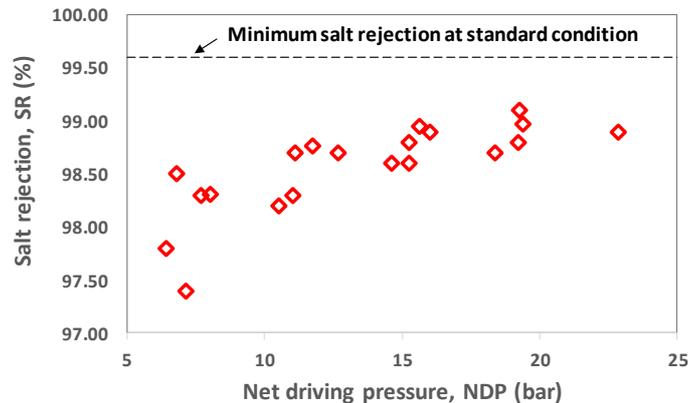
Figure 4. Salt rejection rate at different net driving pressure, *NDP*
