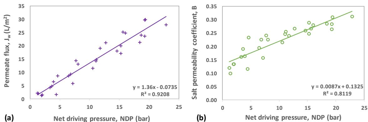
Figure 5. (a) Permeate flux,  $J_w$  and (b) salt permeability factor,  $B$  at different net driving pressure, NDP
