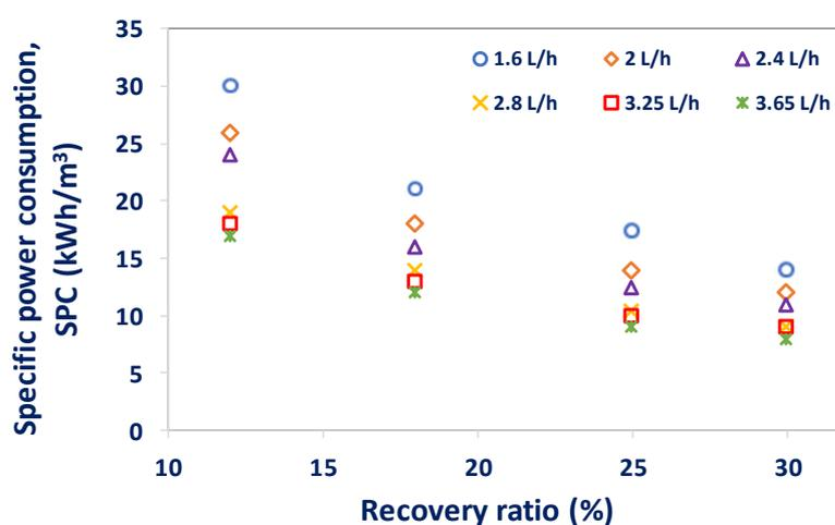
Figure 6. Specific power consumption at different recovery ratios
