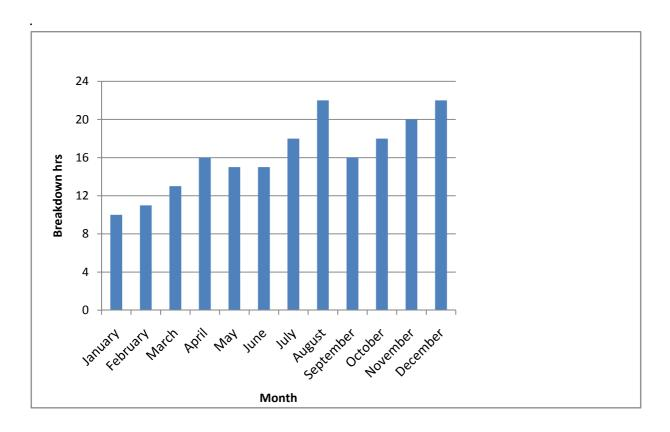
Fig 3.shows monthly breakdown in goliath crane (2010 years)
