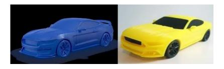
Figure 1. Design and printing of a product based PLA fiber using 3D printer.
