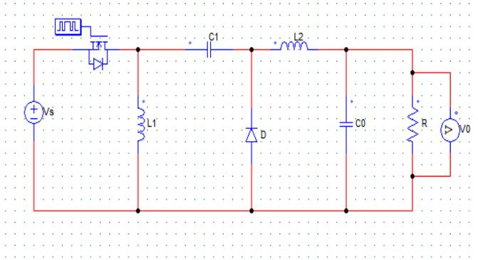
Figure.7Representation diagram of Zeta converter
