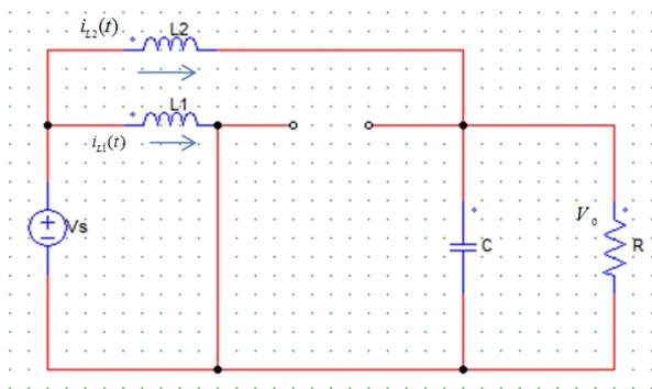
Figure.35 Device 4 Operation of Two Phase Boost Converter
