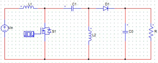
Figure.1 Graphic diagram of Sepic Converter
