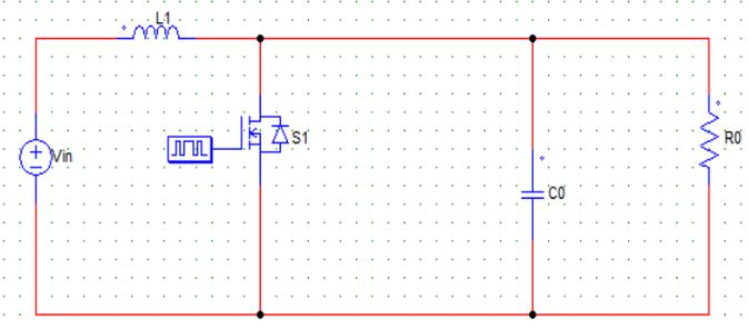
Figure.11 Operation 1 of Boost Converter, i.e., Switch is in ON state
