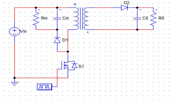
Figure.19 Circuit Diagram of Flyback Converter
