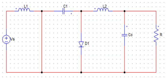
Figure.23 Stage 2 Operation of Cuk Converter, i.e., Switch is in OFF state
