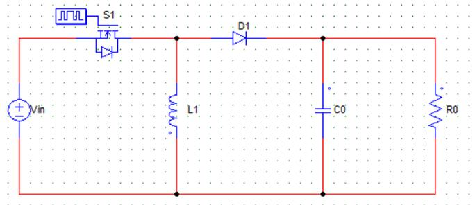
Figure.13 Schematic diagram of Buck-Boost Converter
