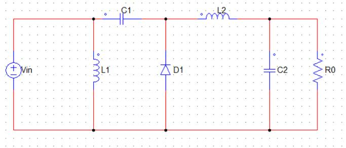
Figure.6 Operation 2 of Luo Converter, i.e., Switch is in OFF state
