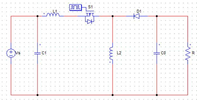
Figure 25. Landsman Converter Diagram
