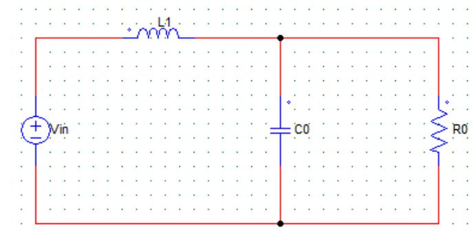
Figure.17 Stage 1 Operation of Buck Converter, i.e., Switch is in ON state
