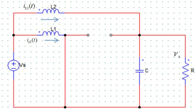
Figure.33 Device 2 Operation of Two Phase Boost Converter
