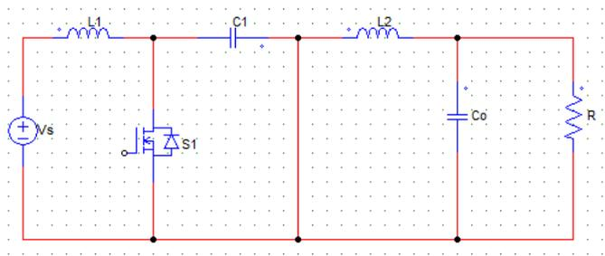
Figure.22 Stage 1 Operation of Cuk Converter, i.e., Switch is in ON state
