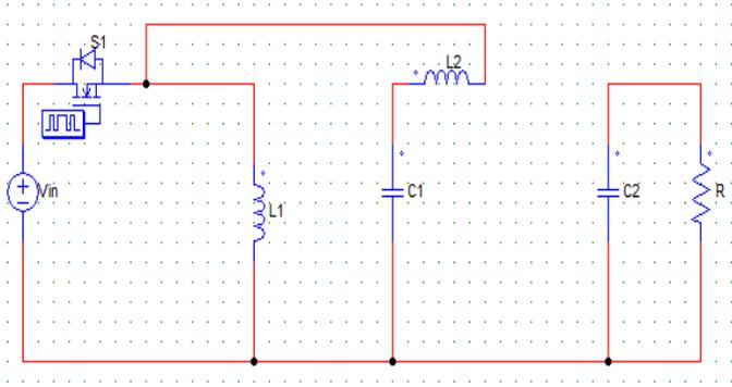
Figure.29 Stage 1 Operation of Ultra-Lift Luo Converter, i.e., Switch is in ON state
