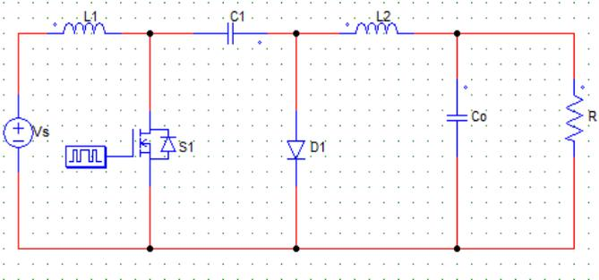
Figure.21 Cuk Converter Diagram
