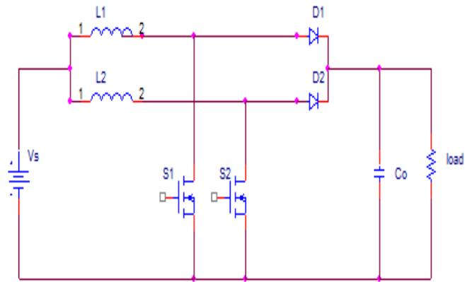
Figure.31 Two Phase Boost Converter Diagram
