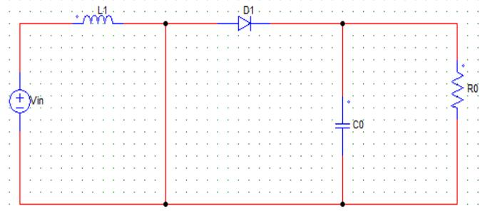
Figure.12 Operation 2 of Boost Converter, i.e., Switch is in OFF state
