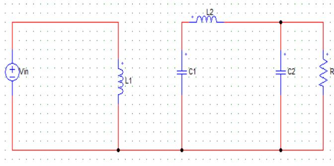
Figure.30 Stage 2 Operation of Ultra-Lift Luo Converter, i.e., Switch is in OFF state
