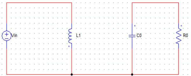
Figure.14 Operation 1 of Buck-Boost Converter, i.e., Switch is in ON state
