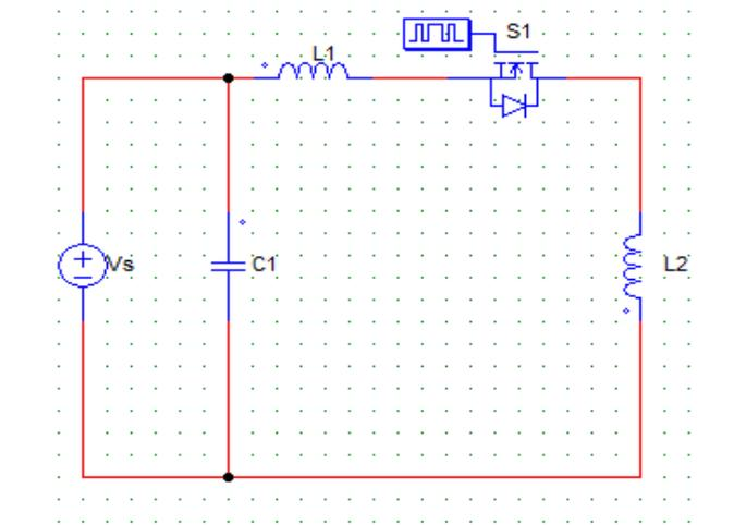
Figure.26 Stage 1 Operation of Landsman Converter, i.e., Switch is in ON state
