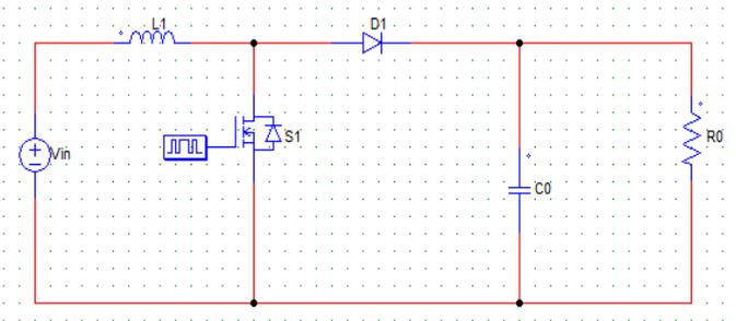
Figure.10 Graphic diagram of Boost Converter
