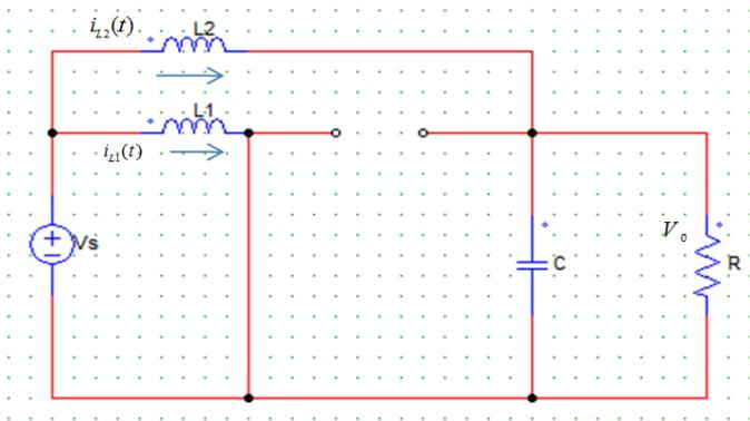
Figure.34 Device 3 Operation of Two Phase Boost Converter
