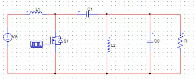
Figure.2 Operation 1 of Sepic Converter, i.e., Switch is in ON state
