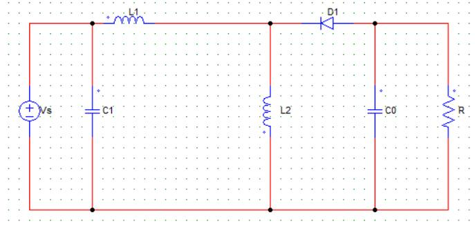
Figure.27 Stage 2 Operation of Landsman Converter, i.e., Switch is in OFF state
