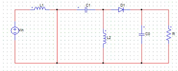
Figure.3 Operation 2 of Sepic Converter, i.e., Switch is in OFF state
