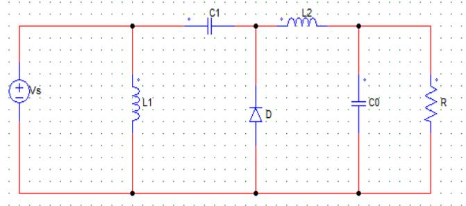
Figure.9 Operation 2 of Zeta Converter, i.e., Switch is in OFF state
