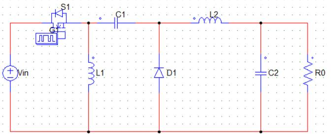
Figure.4 Graphic design of Luo Converter
