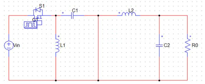
Figure.5 Operation 1 of Luo Converter, i.e., Switch is in ON state
