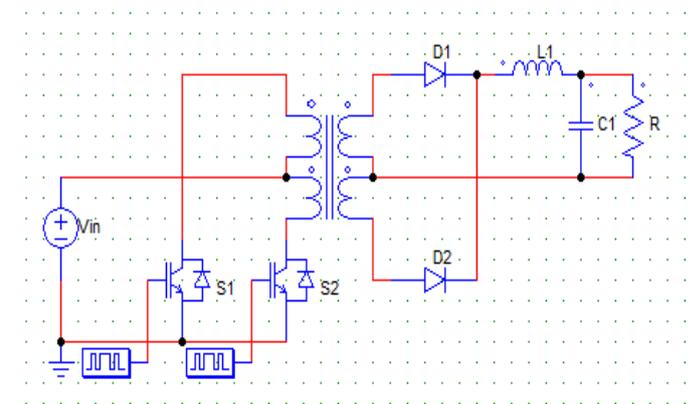
Figure.20 Circuit Diagram of Push Pull Converter
