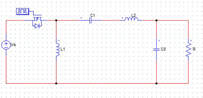
Figure.8 Operation 1 of Zeta Converter, i.e., Switch is in ON state
