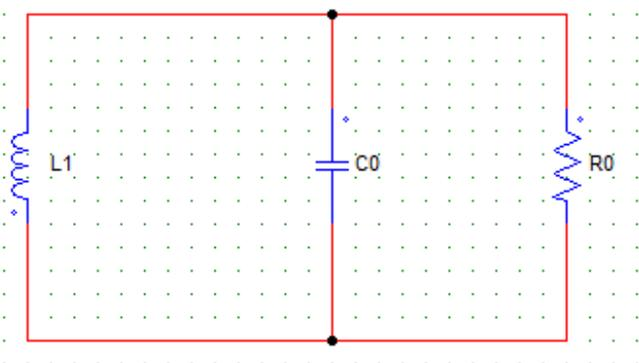
Figure.15 Operation 2 of Buck-Boost Converter, i.e., Switch is in OFF state
