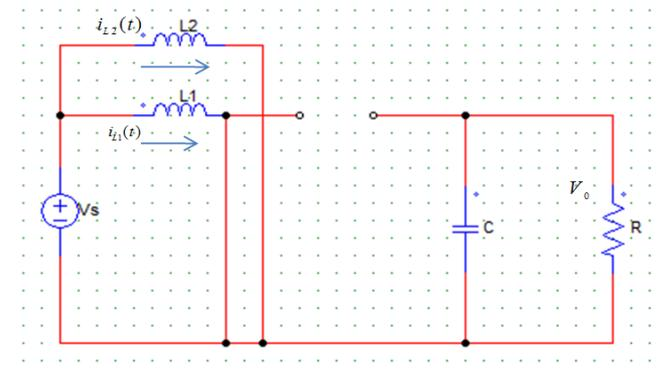
Figure.32 Device 1 Operation of Two Phase Boost Converter
