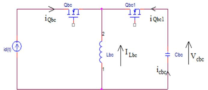
Figure. 36 Equivalent Circuit of Bidirectional DC-DC Converter.
