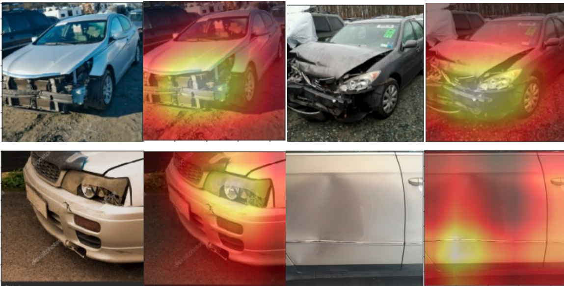
Figure 4: Examples of CAMs, few images of Damaged Cars, and their class activation maps with them. We observe that the damaged regions of the images are often highlighted. Apart from this, similar observations are recorded in other samples.
