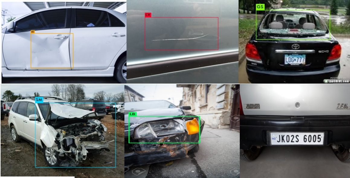
Figure 5: Sample Images of Damage Detection via YOLOv3
