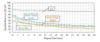
Fig. 6. Sensible heat loss amount by thermal manikin.
