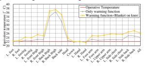
Fig. 7. Equivalent temperature by thermal manikin.
