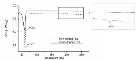
Fig. 5. DSC thermogram of electrosprayed drug-loaded PCL particles (drug: insulin and PTX)
