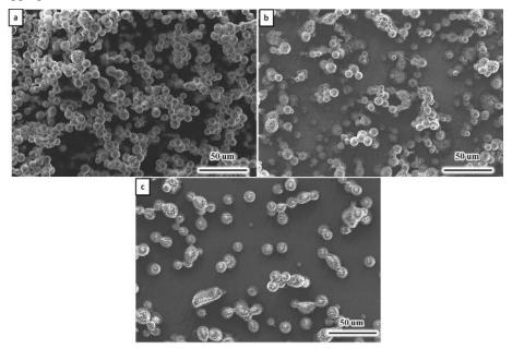
**Fig. 3.** SEM micrograph of drug-loaded PCL microparticles; 4.5% PCL in DCM, applied voltage 18 kV, gauge 20G, collecting distance 21 cm, flow rate 1.2 ml/h with (a) no drug, (b) 15% PTX in PCL particles and (c)15% insulin in PCL particles (w/w).
