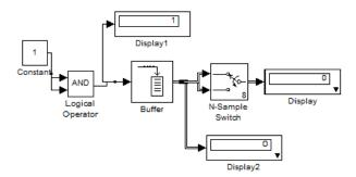
**STEP 5:** Simulation runs for 0.5s and we get desired outputs in the appropriate display box.
