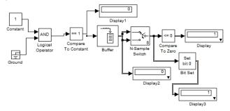
**STEP 3:** Simulation time 0.5s. System ends at the "Display 2" block. Our system works till final output. We get better output.
