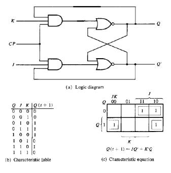
Figure 5: JK Flip-Flop's Operating Table
