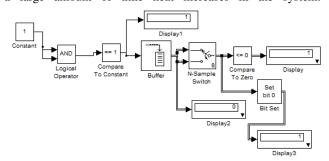
Logic gate induces propagation delay. So, we can also use flip-flop type switch/latch for better performance improvement. Latch has a problem of giving transient output while input changes. Not only transient output, latch has delay incurred due to operation [5]. So, we can check the current and previous output from the operation of Flip-Flop. JK Flip-flop is good for this case of keeping current and previous state change. Operating table of JK Flip-flop is illustrated in Appendix.
