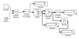
**STEP 4:** Simulation Time 0.05s. System give simulation's output till the "Display1" block output. Rest of the system gives default output. This system needs much area in fabrication and because of digital blocks of comparison, it gives default wrong output. As many blocks need to active for a large amount of time heat increases in the system.
