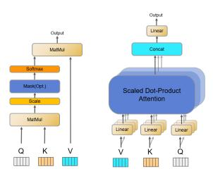
Fig. 1. The scaled dot-product attention model on the left, and the multi-head attention model on the right consists of several parallel attention layers.
