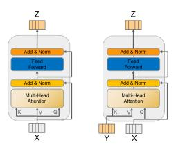
Fig. 2. The left side is the self-attention with multi-head attention as the main structure, and the right side is the guide-attention that introduces the dual modalities of text and images.
