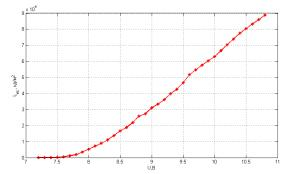
Fig. 1. Calibration curve for sourse brightness depending on the voltage on the LED at  $L_{ad}$  = 54 cd/m<sup>2</sup>
