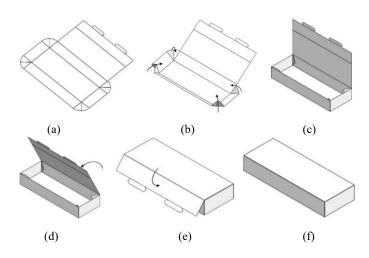
**Fig. 3.** Folding process of egg tart carton. (a) flat cardboard (b) folding four flaps (c) complete folding flaps(d) folding cover panel, (e) folding front panel (f) folding tongue.
