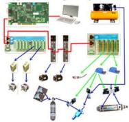
Fig. 12. control system connection diagram of packaging machine.
