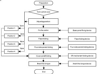
Fig. 4. The workflow of the packaging machine.
