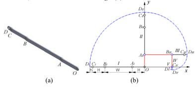
Fig. 9. Theoretical trajectory of cover panel
