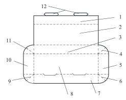
**Fig. 1.** The flat structure of customized egg tart carton (1. front panel, 2.cover panel, 3.rear panel, 4. right rear flap, 5.right panel, 6.right front flap, 7.front inner panel, 8.base panel, 9.left front flap, 10.left panel, 11.right rear flap, 12.tongue)
