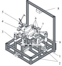
**Fig. 5.** Three-dimensional model of egg tart carton packing machine. (1. base support device, 2. adjustment device, 3. flaps folding device, 4. carton, 5. cover panel folding device-5R mechanism, 6. four side panels folding device, 7. cover panel folding device, 8. control system, 9. tongue guide device)
