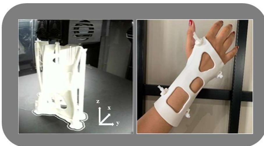
**Figure 1.** 3D printing of arm splint.
