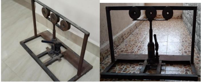
Fig. 7 – Experimental Setup Of Elastic Material Bending Machine.
