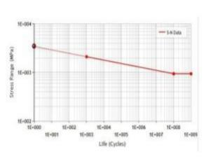
Fig. 6 – S-N Diagram of Structural Steel
