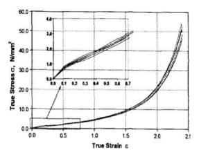
Fig. 5 - Stress & Strain Relation of Polyurethane Rubber
