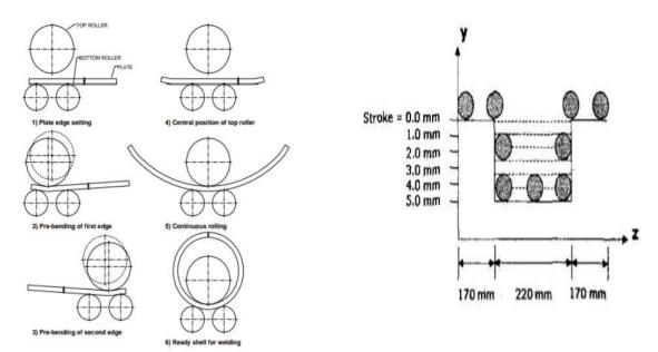
Fig.-1 Pulley sequence for fixed upper pulley gap
