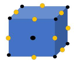
The unit cell of CaTiO3 is seen as an example of the perovskite structure shown above in this diagram. The presence of Ca2+ is shown by black holes at the cube's corners. The yellow holes in between the two Ca2+ ions represent O2-.
