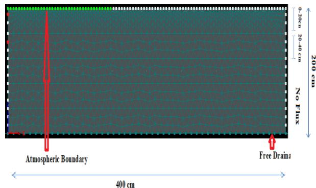
Figure 1: Geometric domain of HYDRUS-2D modeling with observation nodes, and boundary conditions for soil-water
