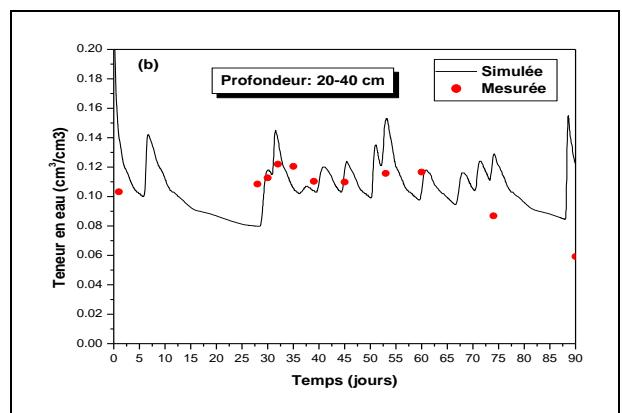
Figure 2: comparison of numerical simulations and experimental values of the volume water content at the depth scale: (a) :0-20cm et (b) :20-40cm.
